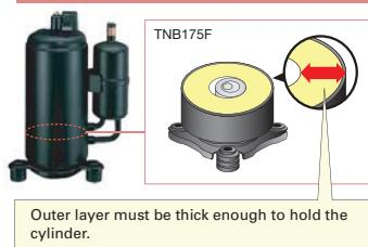
Compressor fixed using Heat Caulking Fixing Method
